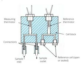
The reference gas chamber, with inlet and outlet openings drilled into the chamber from the base, may be open or sealed. The cells in which the thermistors are mounted are deadened so the sample gas enters only by diffusion, minimising the effect of sample flow variations. In addition, the entire cell-block assembly is maintained at a constant optimum temperature through two heaters and a control thermistor which are located in the cell-block assembly.
